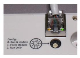
To address LP283W connect the LCD and set the "rotary switch" in position "1" to access the setup menu.
