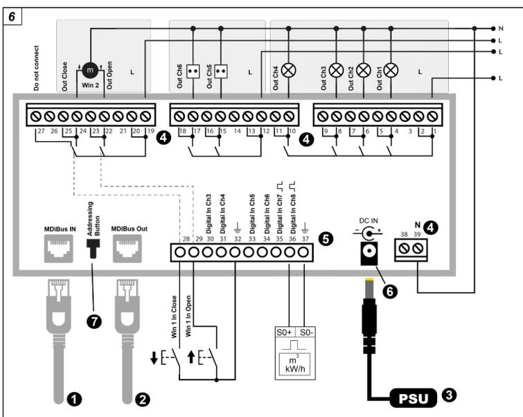
**iOW88 – 8 ch ON/OFF + 8 ch digital input**
